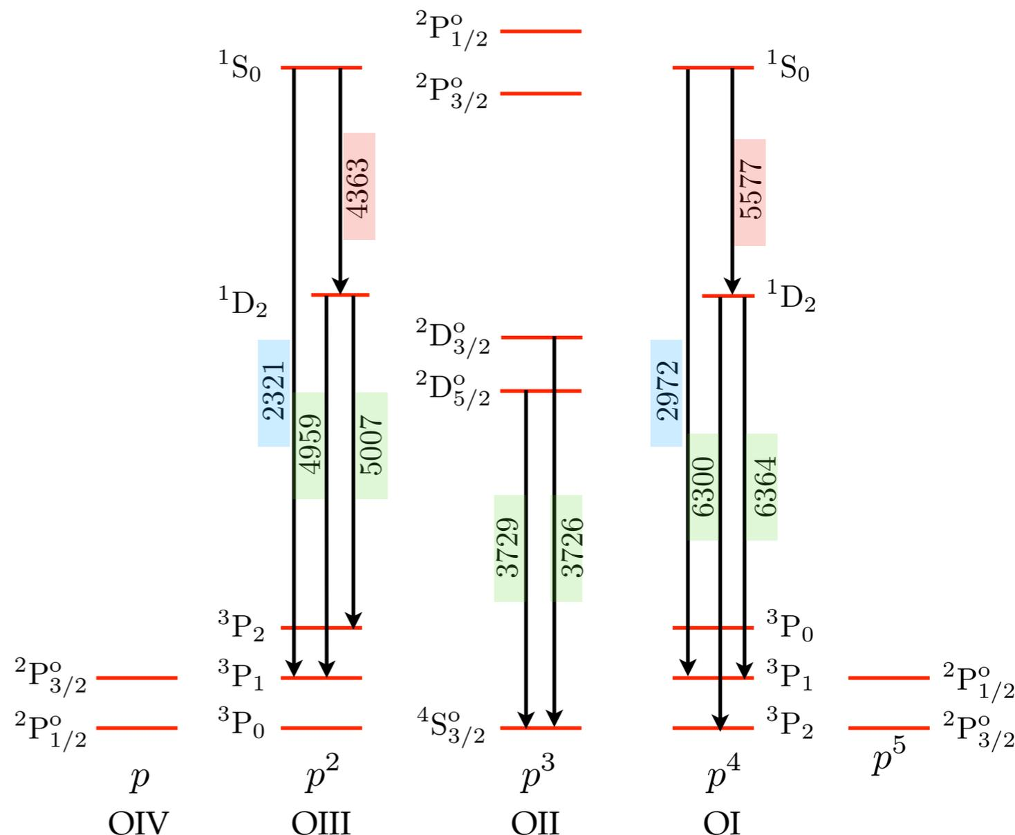
The term structure for the ground configurations with  $p$ ,  $p^2$ ,  $p^3$ ,  $p^4$ , and  $p^5$  outermost shells. (not to scale)
