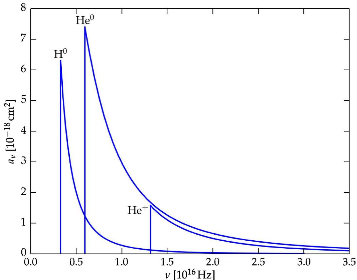
Photoionization cross section for hydrogen( $H^0$ ), hydrogenic helium ( $He^+$ ), and neutral helium ( $He^0$ ). [Fig. 4.1 in Ryden]
